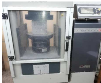
Figure 2. Compressive strength experiment.
