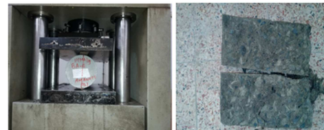
Figure 3. Splitting Tensile Strength Experiment.
